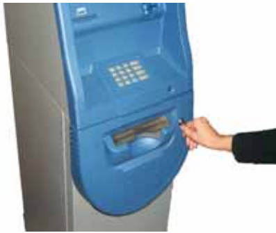
Fig.A-2 Closing the Security Door
