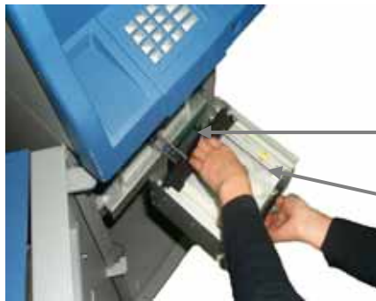
Fig. 5.3a Replenishing the Cash Cassette
