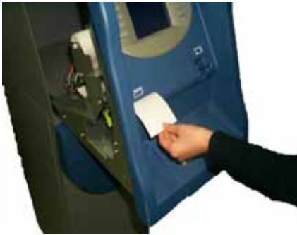
Fig 5.5a Loading the Receipt Paper
