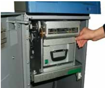
Fig. 5.4 Emptying the Reject Bin
