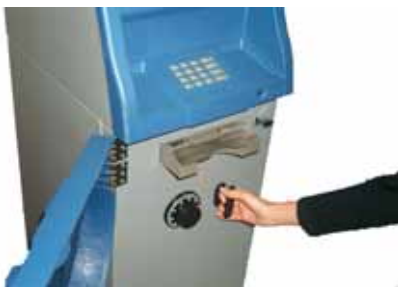
Fig. B-3 Replenishing the Cash Cassette
