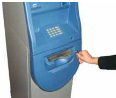
Fig.5.1b Closing the Security Door
