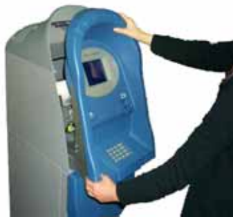
Fig. 5.2a Opening the Front Panel
