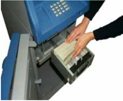
Fig. 5.3a Replenishing the Cash Cassette
