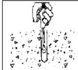
Blow or vacuum out dust/debris.
