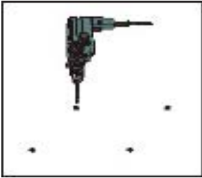
Drill anchor holes
